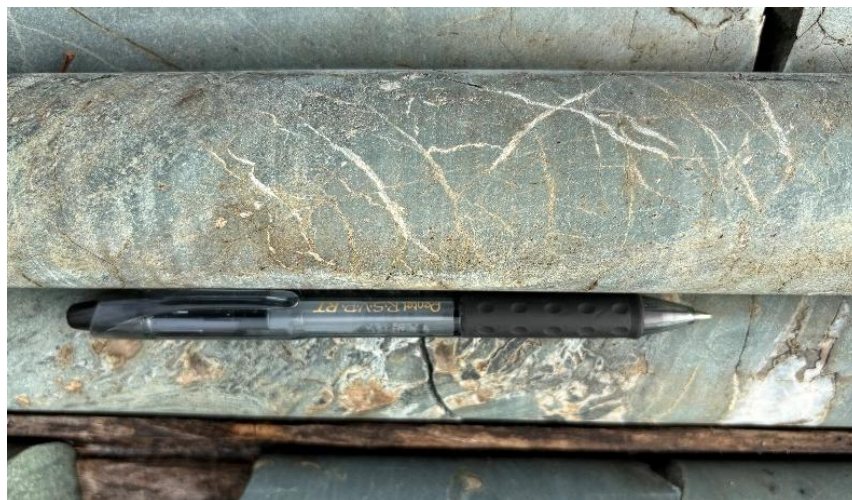
Figure 12.5 Example of Drill Core Intercept Observed Showing Millerite (in pen area) Flanked by Lizardite
